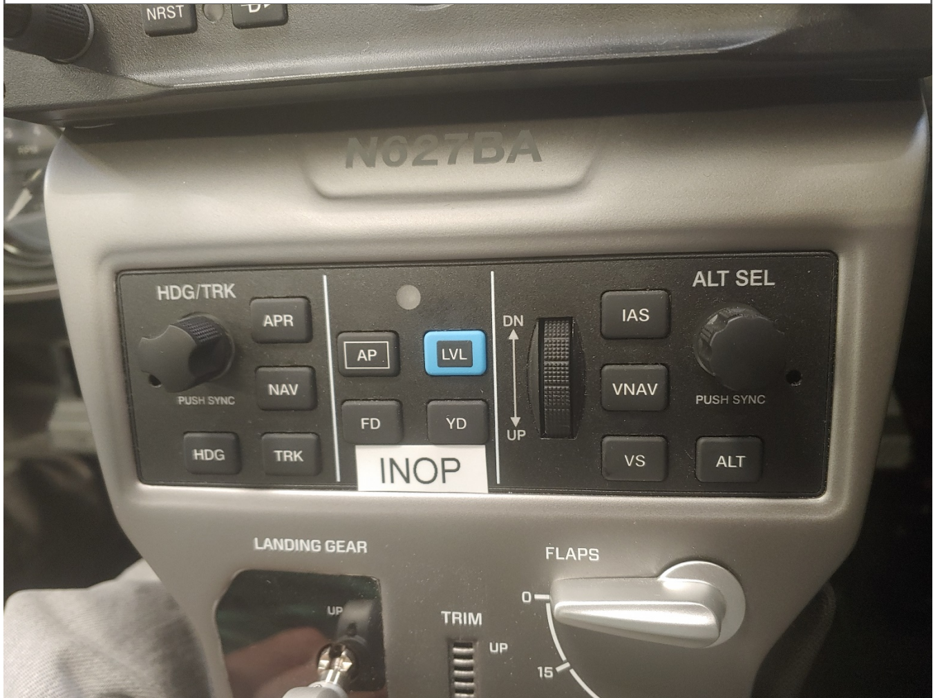
Figure 8: "INOP" label installation
