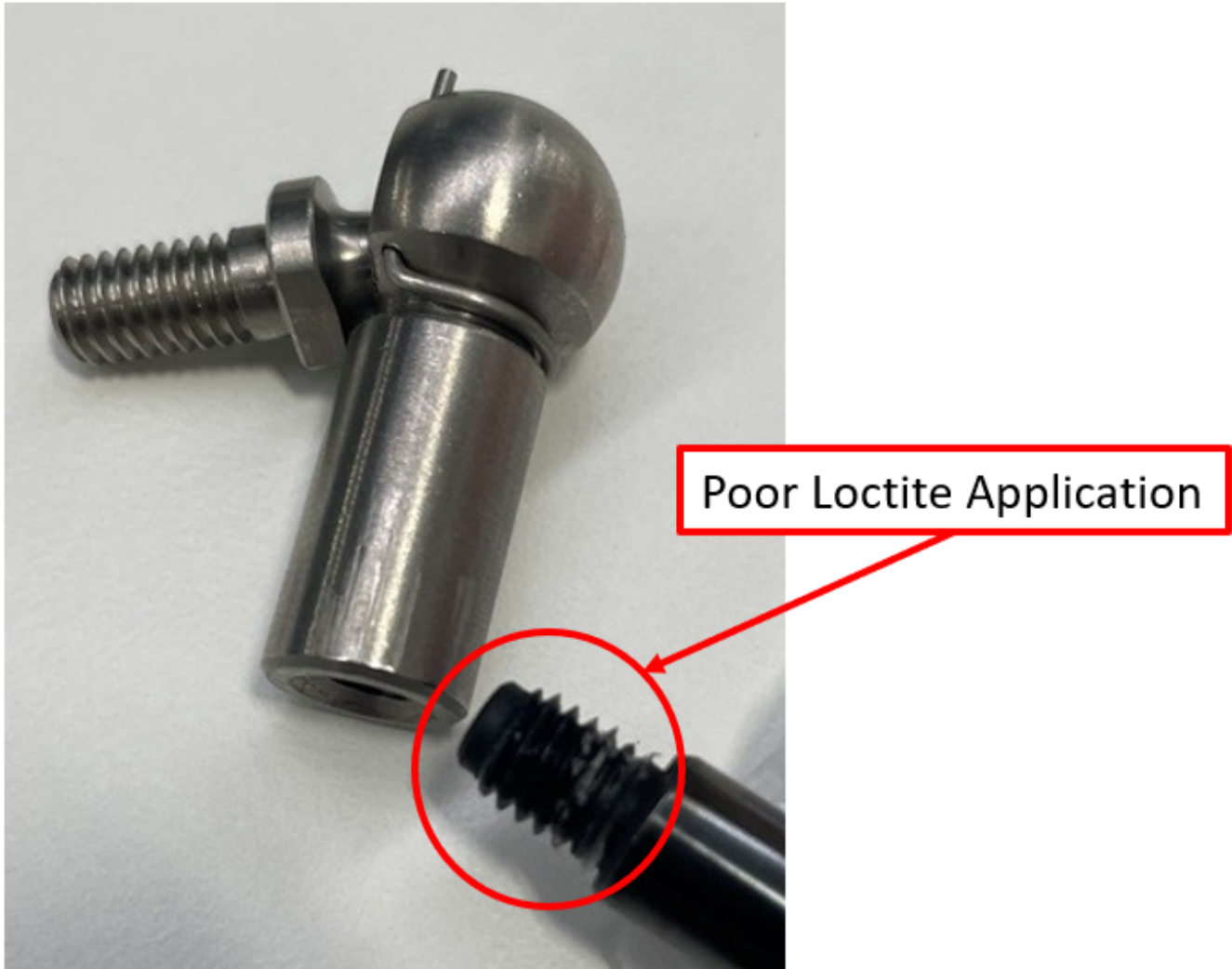
Figure 2 Poor Loctite Application
