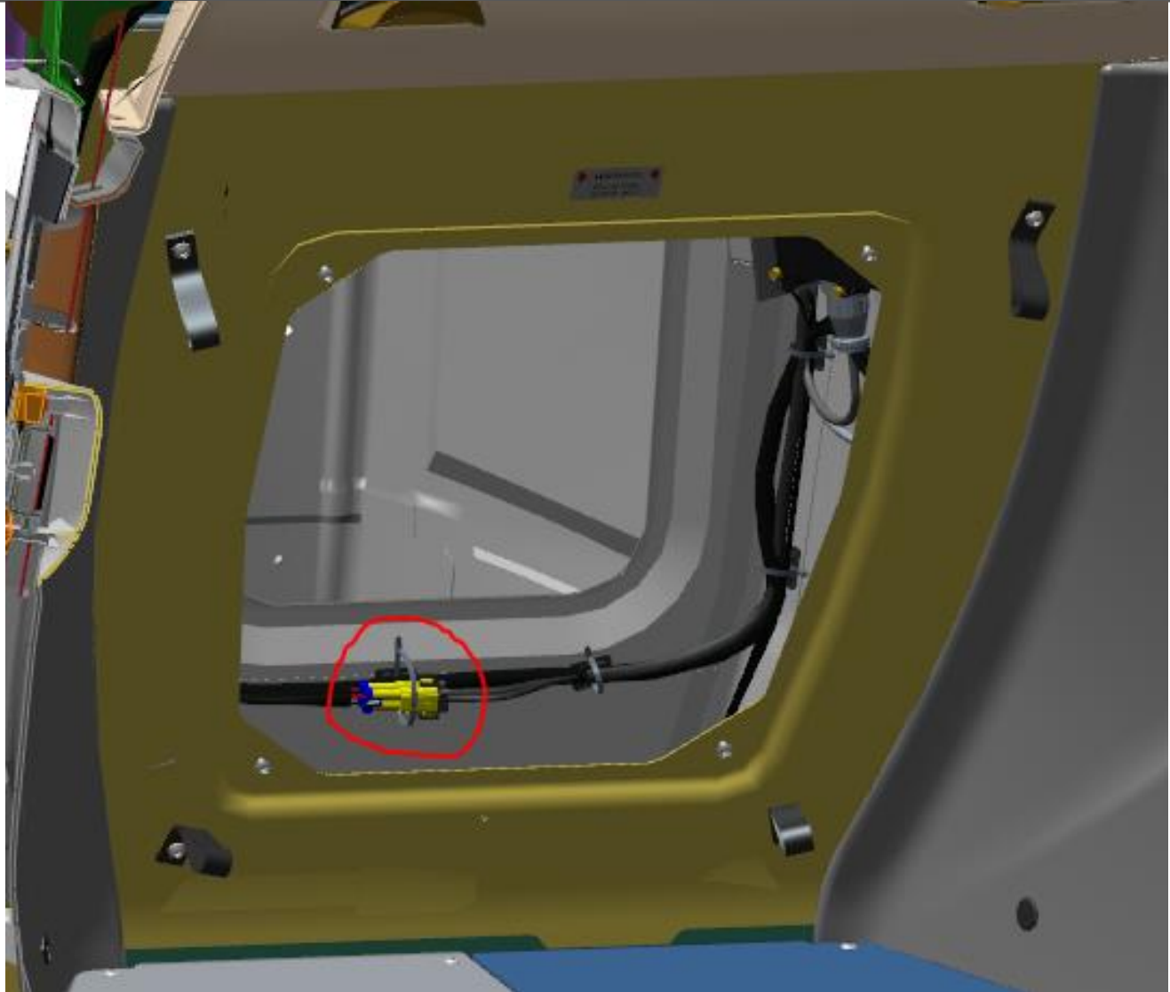
Figure 8: Fuel Pump Extension Connectors Location
