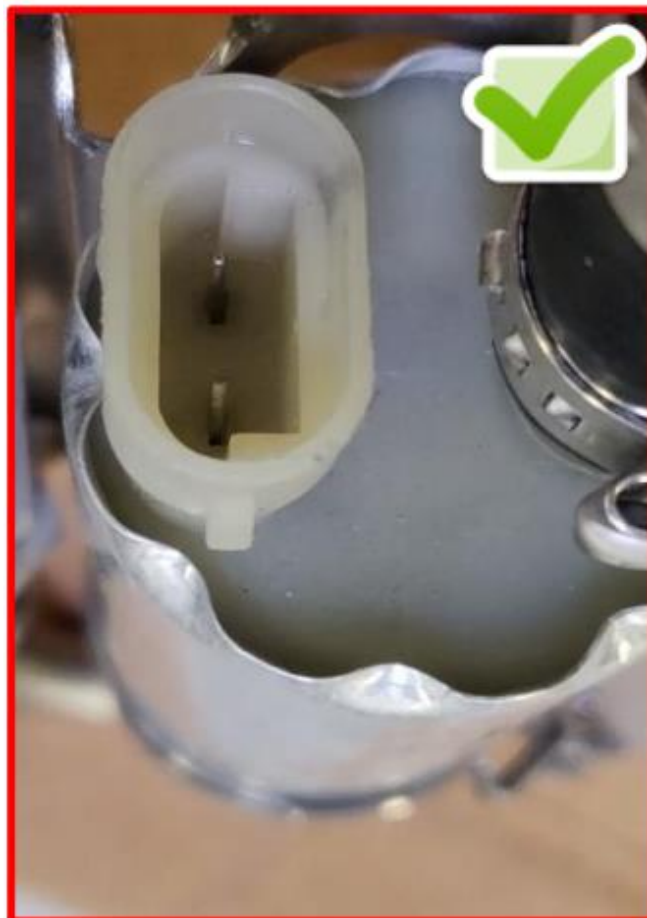
Figure 4: Fuel Pump pins must be straight
