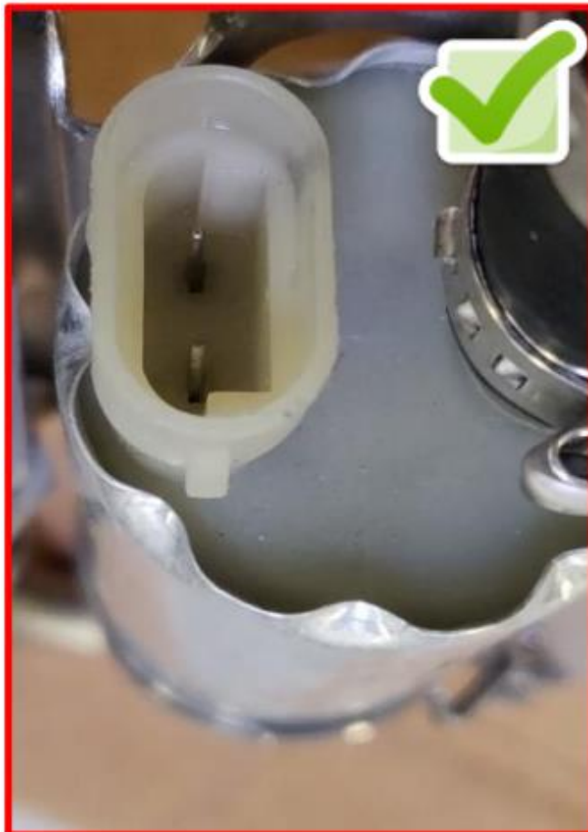
Figure 3: Fuel pump pins must be straight
