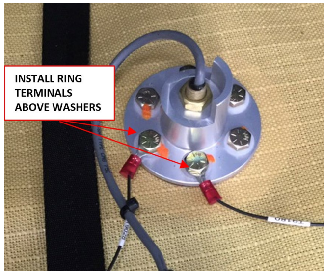
Figure 10 – Fuel level sensor orientation.
