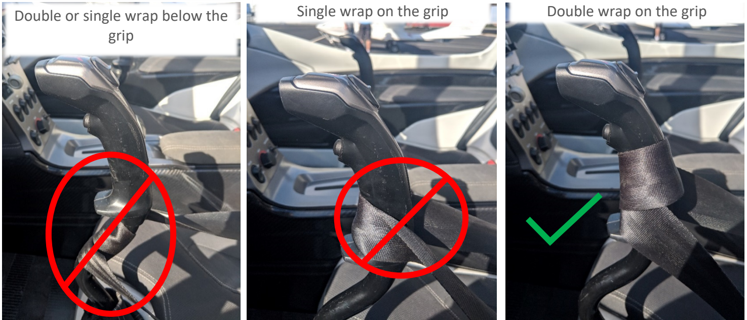
Figure 2: Seatbelt should be double looped around control stick grip. Single looping around grip, or double looping around stick shaft will not properly secure control surfaces.
